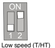
Dip switch 1 should be in the 'OFF' position (T and HT models only).
