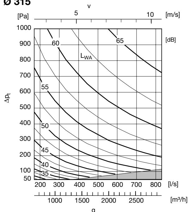
The grey area in the graph shows the minimum pressure drop needed for the product to start working. Even if the damper blade is fully open you get this pressure drop over the product.
