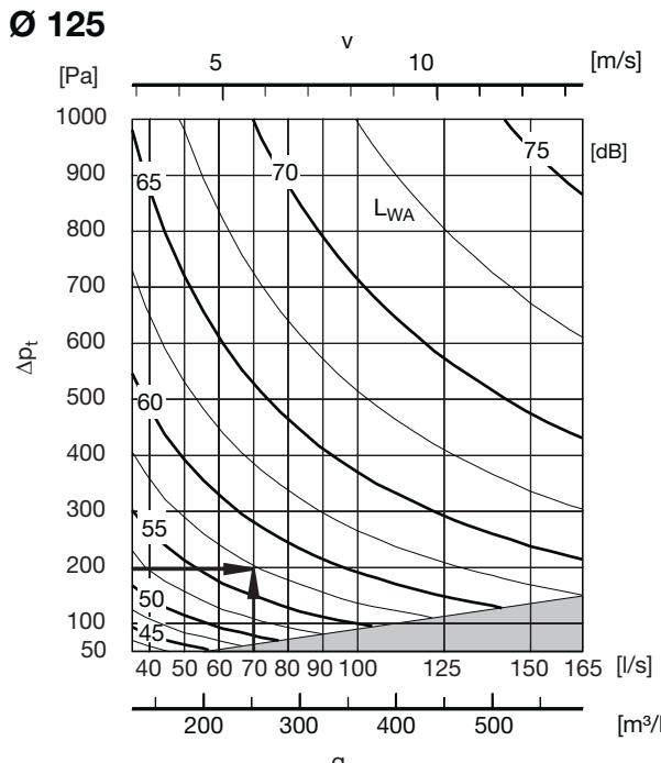
The grey area in the graph shows the minimum pressure drop needed for the product to start working. Even if the damper blade is fully open you get this pressure drop over the product.
