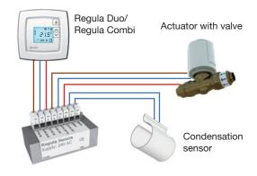
Schematic showing how to connect Regula Secura.
