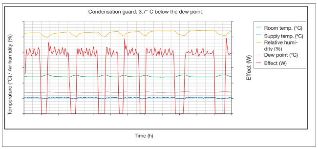
The diagram shows a control sequence where the water temperature is 3.7°C below the dew point. Throughout the whole process, the control centre asks for cooling. It can be seen how Regula Secura controls using the ON/OFF feature.
