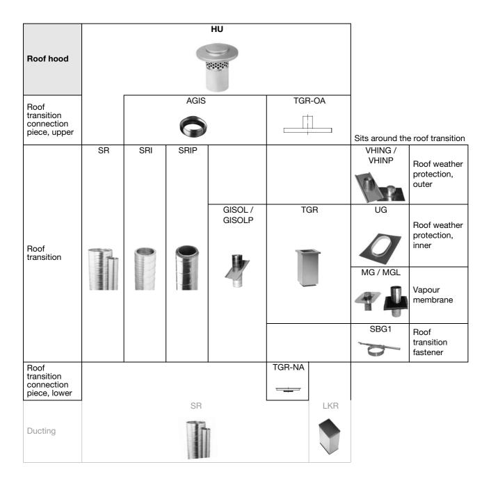
This diagram shows pricipally all possible combinations of how the products can be joined together. Normally only one alternative is chosen and sometimes some options are omitted.
