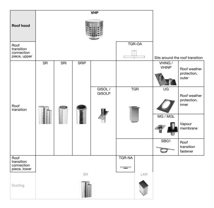
This diagram shows pricipally all possible combinations of how the products can be joined together. Normally only one alternative is chosen and sometimes some options are omitted.
